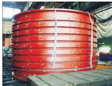
The segments are screwed to thickened side plates of disks using the analogous technology as that used with connecting frictional disk halves (hydraulically tightened screws with defined axial pre-stress). Mutual location of individual segments is stabilized by the help of locks of groove and tongue type. To every brake disk, sensors automatically checking the extent of its axial run-out are installed on mounting.
